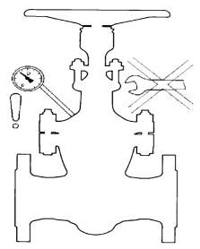
Spring loaded stuffing boxes must also be checked for tightness during operation, and tightened as necessary (see point 4.1). It should be noted that the stuffing box must seal without a major increase of friction at the spindle. We recommend that regular checks be carried out during operation.
