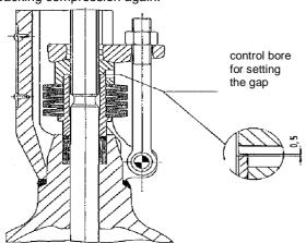
After this maintenance, another 100 cycles of the valve are possible, staying within the leakage rates determined by TA-luft. The next shutdown should then be used to exchange and reset the packing. For this replacement we recommend that the new packing be installed and precompressed with a proper tool (f.e. a copper bar) following above mentioned and general maintenance rules.
