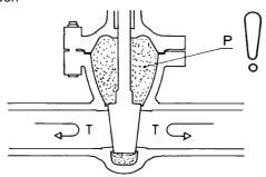
Reference literature states that bolted bonnet flanges can solve the overpressure problem by using connecting bolts which elongate to leave a gap between the flanges that in turn relieves the pressure. Practical experience has confirmed this theory, although it is essential to note that a bolted bonnet flange which leaks in this way can blow off uncontrolled in all directions and cause a danger and/or damage the valve.
