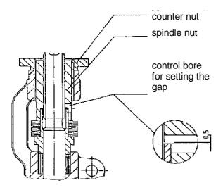
Persta recommends to follow up the frequency of operation. After  $\pm$  500 cycles, the stuffing box should be retightened as follows.
