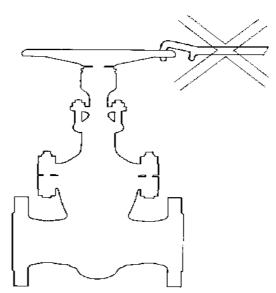
VALVES WITH HANDWHEELS MUST ONLY EVER BE MANUALLY OPERATED. THE USE OF BARS OR PIPES TO INCREASE LEVERAGE CAN DAMAGE THE UNIT AND CAUSE AN ACCIDENT THROUGH SLIPPAGE OR FAILURE, AND IS NOT PERMITTED.
