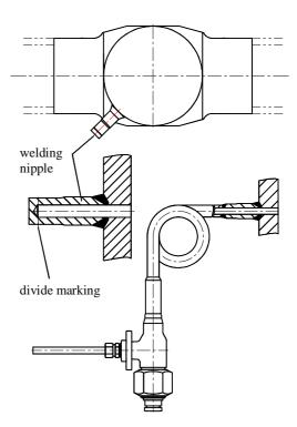
If these valves are ordered with this closed stud and a safety device, we normally deliver the piping and safety device not fitted to the main valve, because we are unknown about the location. The welding of these parts has to be carried out by qualified welders who have experience with the material. In regards of the proper function and direction of the safety valve you have to follow the operation and maintenance instructions.
